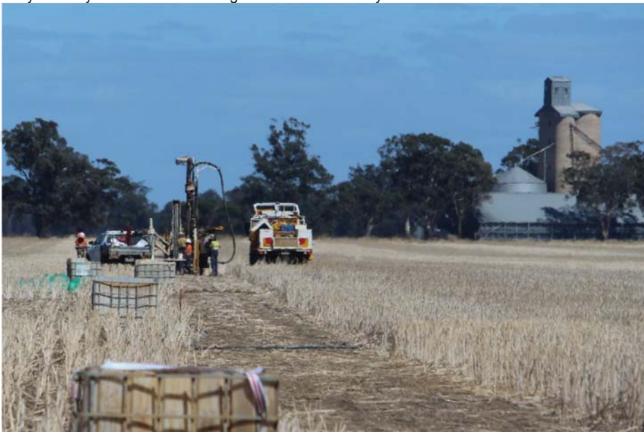
Figure 3 – Air Core drilling underway in Barrabool Tenement.
