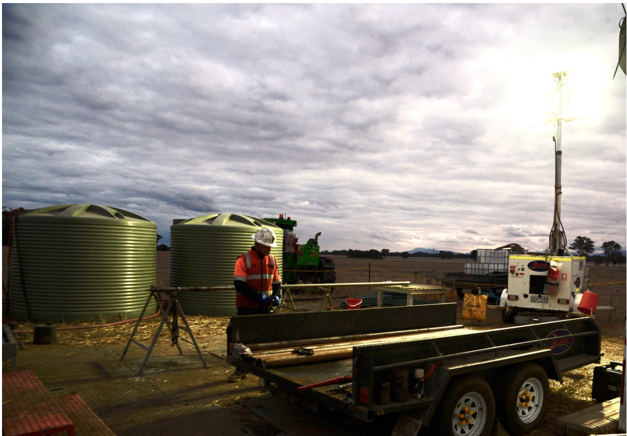
Fig2. Preparing to orient inner tube prior to core removal, Rig1275, Wildwood.
